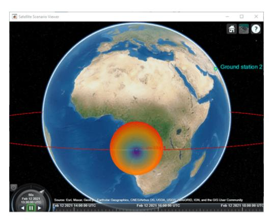
Point the satellite at the ground station. The pattern rotates to reflect the new orientation of the antenna.
